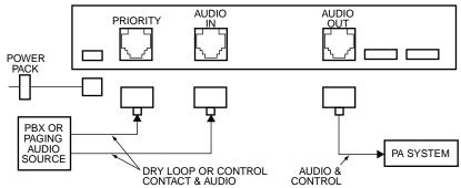
The FE-3S is typically installed between the telephone system, or paging microphone console and the paging system amplifier(s), as shown. It interfaces with the paging controller in a zone paging environment, and with the amplifier in a single-zone installation.
